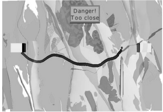
Figure 3. Screen shot of mine planning geological scene showing rock layers and tunnel route being drawn.
