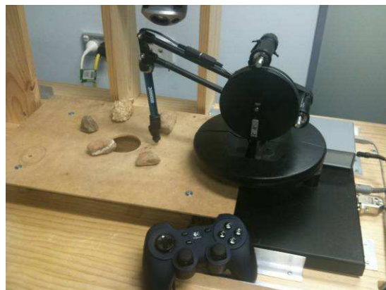
Figure 3. Miniature robotic arm. Also showing joystick interface.
