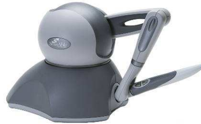
Figure 2. Sensable Phantom Omni haptic device
