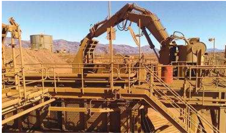
Figure 1. A mining rock breaker
